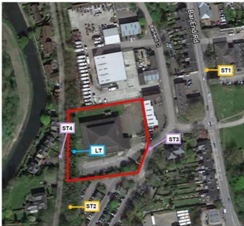
Figure 2. Approximate noise measurement positions overlaid onto a Google Earth satellite image
